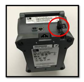
• Using a Philips-Head #2 screwdriver, remove the three screws that attach the power supply assembly to the bottom of the printer and then pull the power supply away from the printer.
